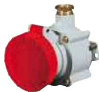
UNAV 2166 socket-outlets in marine grey painted brass with UNAV 1948 cable gland 50-60Hz IP66
