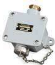
UNAV 1435 socket-outlets in marine grey painted brass with terminal block and UNAV 1948 cable gland 50-60Hz IP66
