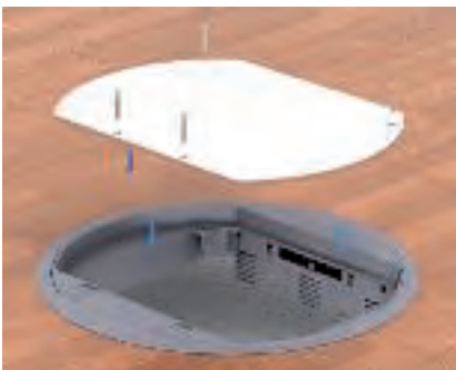
Adjust of the floor covering recess to 12 mm Slacken the 4 lid screws and remove the inserted 7 mm spacer frame. Screw the sheet steel lid on again.
