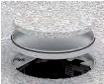
Laying the floor covering in the RKR cassette Lay the floor covering in the cassette and stick it down. Seal the remaining gap between the floor covering and the cassette with suitable materials.
