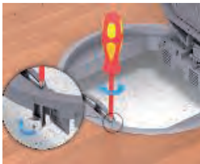
Universal fastening, duct mounting On screwing in, the retaining profile automatically turns outward. It grips under the mounting lid.
