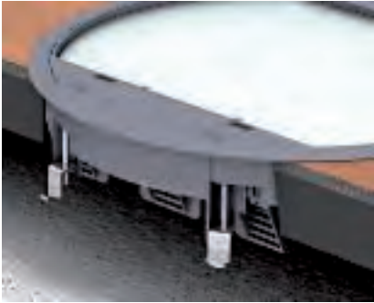
Universal fastening, raised floor mounting, s \geq 47 mm Slacken the retaining profile from the screw and turn it round. Turn the screw back into the retaining profile. In this position, the clamping range is 37 to 75 mm.
