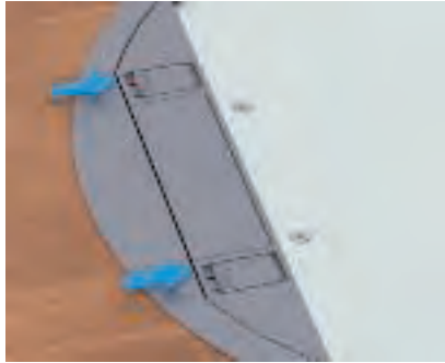
Opening of the hinged lid for GESR9-2U Actuate both lid sliders. The fitters push the hinged lid upwards. Lift the lid using the cord outlet.
