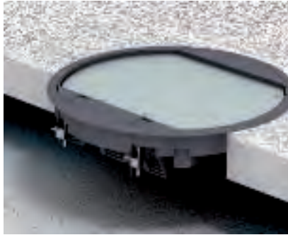
Universal fastening, cavity floor mounting On screwing in, the retaining profile automatically turns outward, locking the service outlet.
