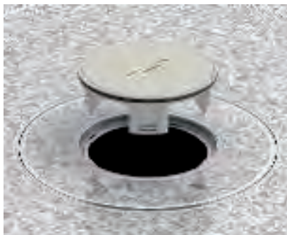
Mounting of tube body Insert the tube body cover into the tube body seat and lower it. Unlock the tube body by turning it to the right and close it flush to the floor.
