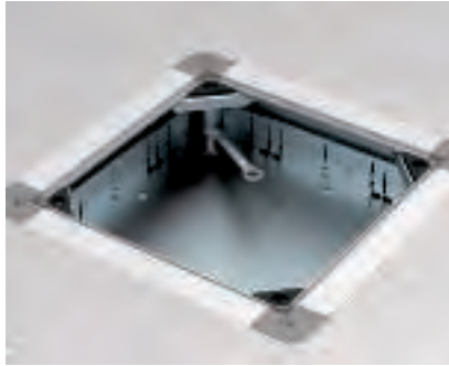
Preparation of an underfloor system Insert the four heavy-duty lid supports in the corners of the underfloor box and adjust them to the required height. Lock the support screw with a locknut.
