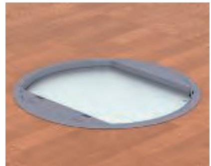
Adjust of the floor covering recess to 10 mm Slacken the 4 lid screws and the inserted 7 mm spacer frame and replace it with the 2 mm spacer bars. Screw the sheet steel lid on again.
