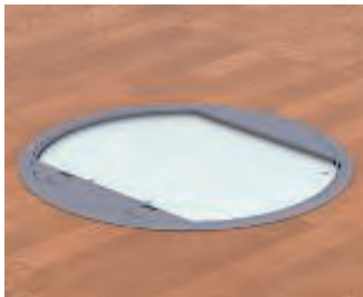
Installation of the hinged cover for GESR round service outlet Slacken the 4 lid screws and the inserted 7 mm spacer frame and replace it with the 2 mm spacer bars. Screw the sheet steel lid on again.
