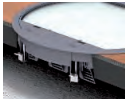
Universal fastening, raised floor mounting The clamping range of the retaining profile is suitable for raised floor plates of a thickness of up to 45 mm.
