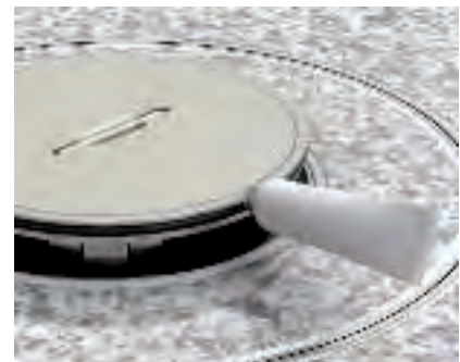
Cleaning of the seals To complete the mounting work, clean the interior of the cassette and the seals of the cassette and tube body. Apply Vaseline to the seals (contained in the scope of delivery).
