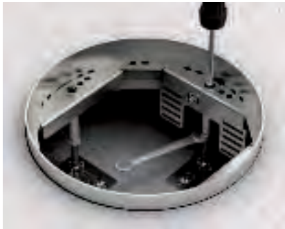
Adjustment of the cassette height Adjust the cassette frame to the top edge of the floor covering. Secure the height adjustment of the height-adjustment screws with lock-nuts.
